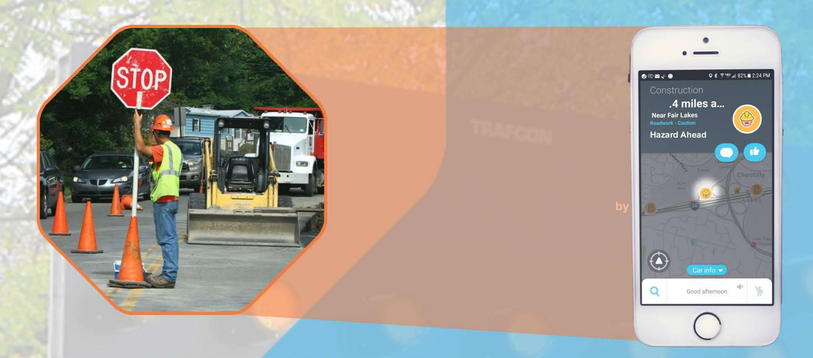
The ConnectedTech Flagging Baton provides the GPS location and the expected delay that is being created by the paddle operator and passes it to the navigation devices miles before the road work allowing drivers the option of choosing alternate routes avoiding the minutes idling and increasing safety for all.
